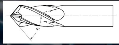
This tool is 7.0° ICL (3.5° per side, called from centerline with a .187 tip diameter and radius)
